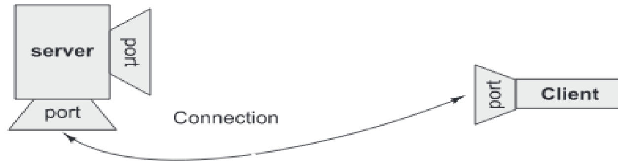
[b]: session established with temporary ports used for two way communication.
